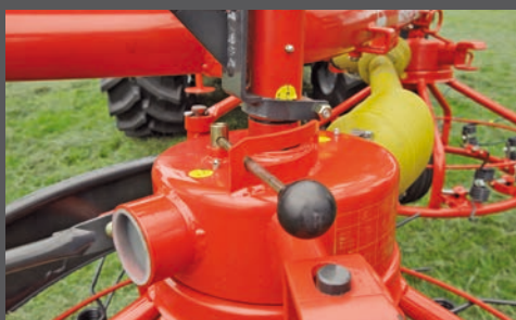
Lever for reversing rotor rotation and instruction decal (Haybob 360)
