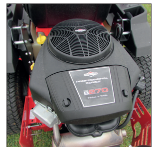
Briggs & Stratton motor 27 hk Intek™ 8270 OHV V-Twin.
