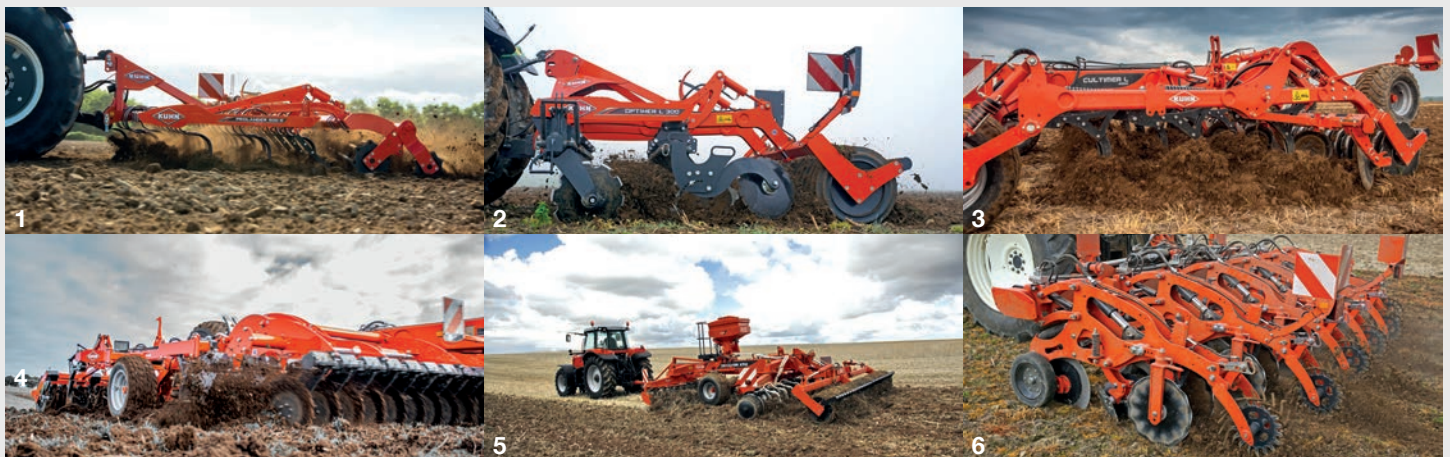
1. PROLANDER vibrating tine cultivator - 2. OPTIMER independent disc stubble cultivator - 3. CULTIMER tine stubble cultivator - 4. PERFORMER tine/disc cultivator - 5. DISCOVER/DISCOLANDER disc stubble cultivators - 6. STRIGER 100 strip till implement
