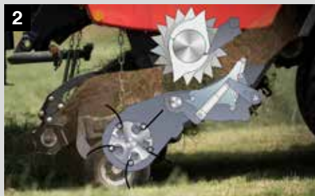
2 Once the PTO is disengaged by the operator, the baler automatically starts the deblocking sequence. First the knives are retracted from the inlet channel, followed by the lowering of the dropfloor system
