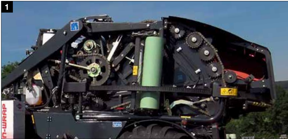
Robust driveline with high quality IWIS chains
