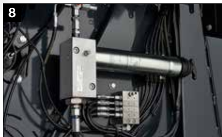
8 Standard automatic greasing system for roller bearings
