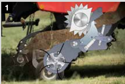
1 When an intake blockage occurs, the operator is informed via an acoustic and visual signal on the control terminal. The intake is protected using the cam clutch protection on the main drive
