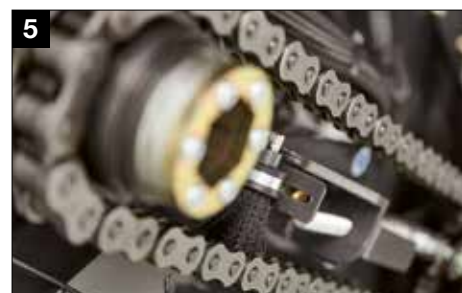
Sturdy and wide oil brushes on the chains ensure perfect lubrication
