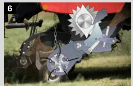
6 After bringing back the dropfloor into position, also the knife bank is brought back into position. The separate dropfloor-knife action ensures a fast and secure process
