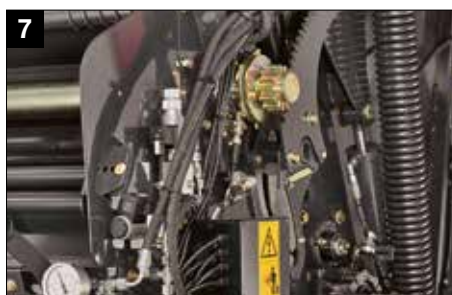
7 Proportional valve for in-cab density control
