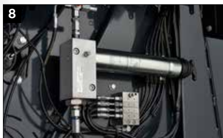
8 Standard automatic greasing system for roller bearings
