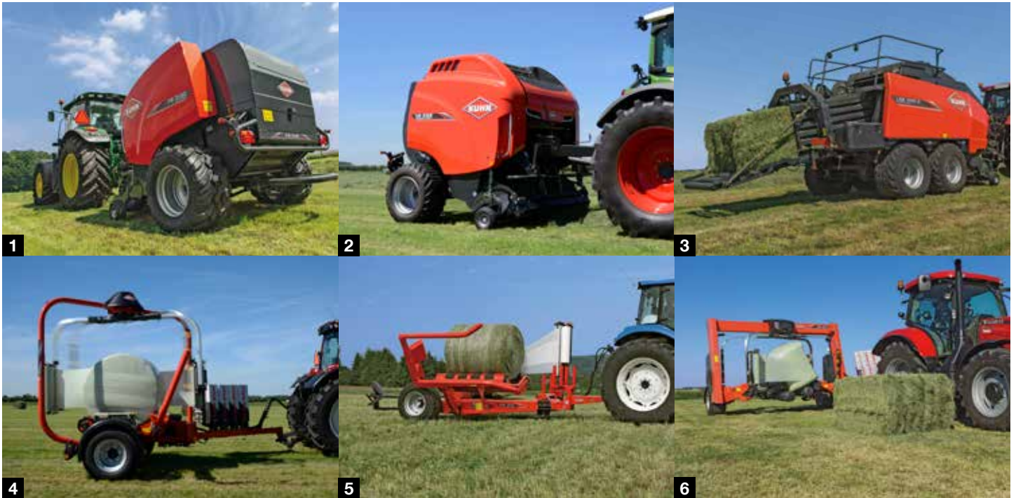
1. Fixed Balers - 2. Variable Balers - 3. Large Square Balers - 4. + 5. + 6. Round and Square Bale Wrappers.
