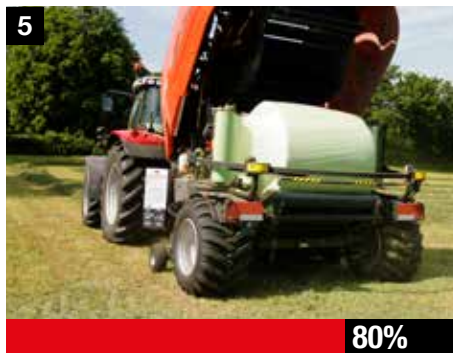
5 80% Unique to the i-BIO is the wrapping ring, with two pre-stretchers. At high speed, the complete bale is wrapped with stretch film, creating a perfect, airtight, seal
