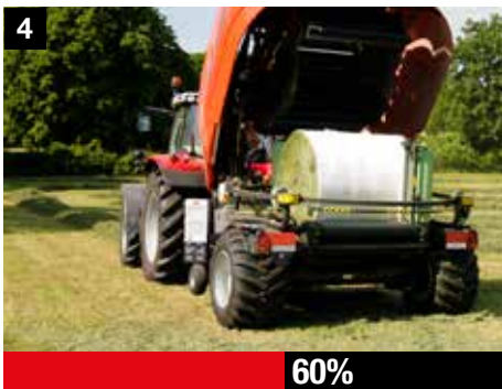
4 60% After the binding cycles, which can either be performed with net or film, the wrapping cycles can start. Thanks to the unique i-BIO design, there is no need for a bale transfer which can help you to save wrapping costs
