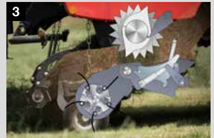
3 After lowering the knife bank and the dropfloor, the operator can re-engage the PTO drive of the machine. Thanks to the lowered dropfloor system, the aggregated crop can be fed into the machine
