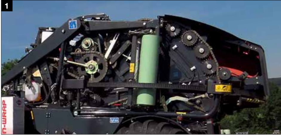
Robust driveline with high quality IWIS chains
