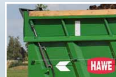
Hydraulic Side wall extension, 300 mm for compost or other light spreading material.
