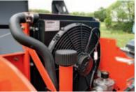
**Q** A 12 kW air-cooled radiator as standard for constant power. All hydraulic components are protected against temperature peaks.
