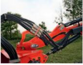
**O Hose routing** designed for optimum protection. All arm hoses are integrated into a protective casing. A swivelling and rotating hose support plate reduces friction phenomena at the pivot.
