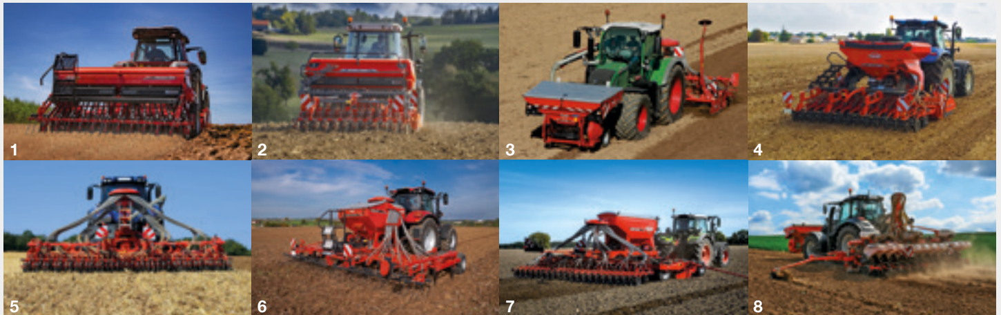
1. Mounted mechanical - 2. Integrated mechanical - 3. With front hopper - 4. Integrated pneumatic - 5. Trailed pneumatic 6. Mounted min-till - 7. Trailed min-till - 8. Precision seed drills
