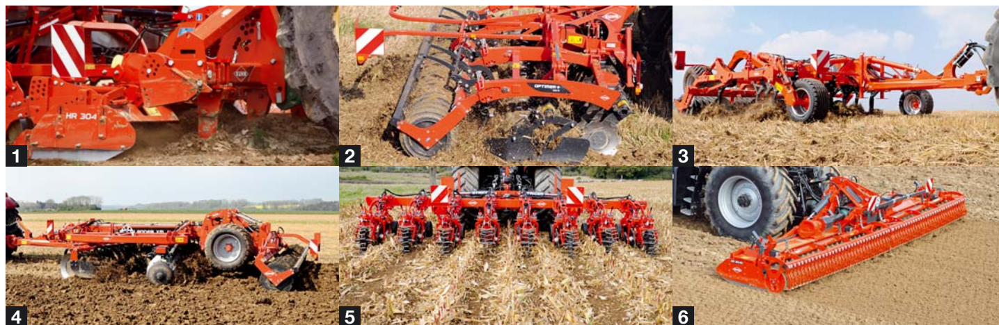
1. Forgrubber - 2. Kompakte tallerkenharver - 3. Stubharver - 4. Tallerkenharver - 5. Strip-tiller - 6. Rotorharver.
